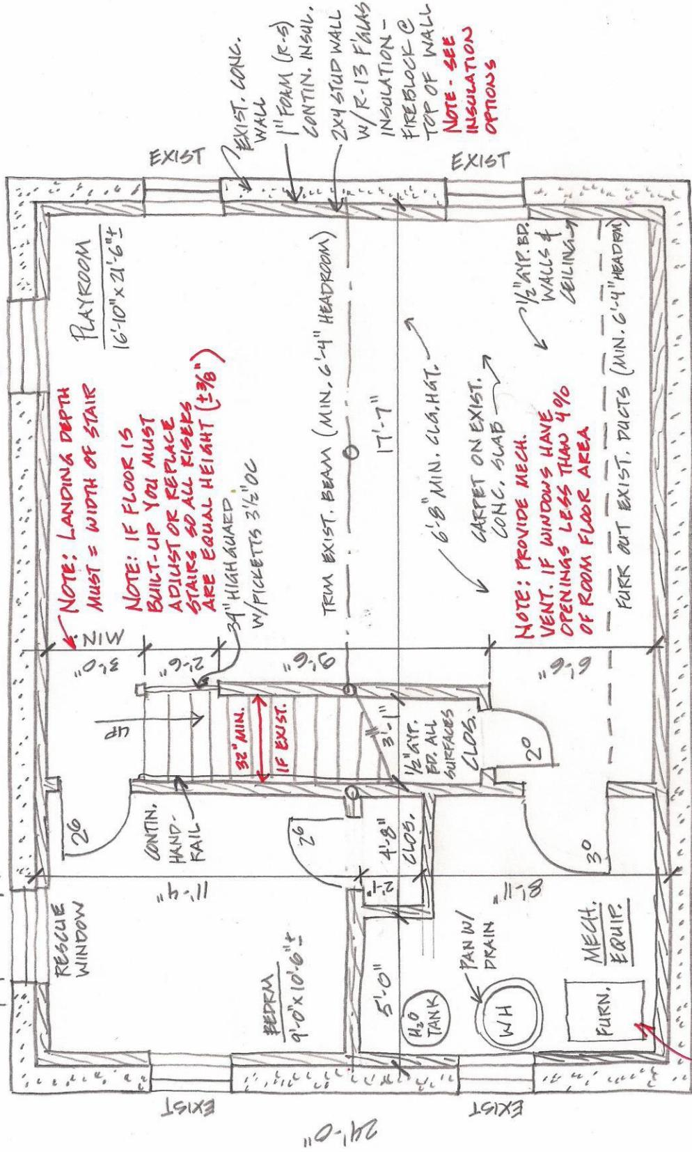
NOTE: PROVIDE COMBUSTION AIR FOR ALL FUEL-FIRED MECHANICAL EQUIPMENT
