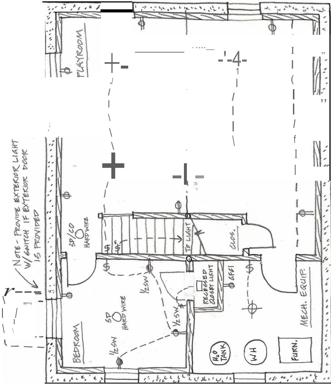
NOTE - ADD BATTERY POWERED SMOKE & CO DETECTORS IN LOCATIONS REQ'D. BY CODE THROUGHOUT HOUSE WHERE NONE EXIST.
